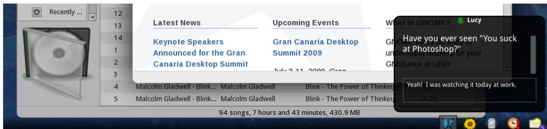
The details mode for a Message Source displays information in a way that is appropriate for that Source. This may involve simply showing an informative message or even allow the user to directly respond to an Instant Message.
