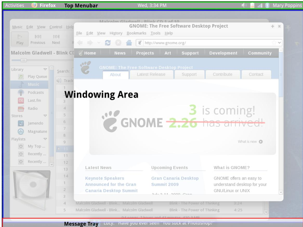
The main scene has three primary, normally visible, areas for interaction: the **Top Menubar**, **Windowing Area**, and **Message Tray**. In addition to these there is another that is not normally visible, the **Activity Switcher** (also known as the Alt-Tab Switcher). We'll now explore each of these in some depth.
